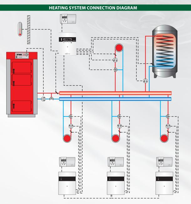
Example of a heating system diagram using the DKMATIC controller with three extension modules DKMZ1: Loop 3, Loop 4, and Loop 5. Without cut-off and safety devices. It is not a replacement for a professional design at the installation site.
