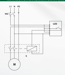
WG - main switch S - contactor M - motor
