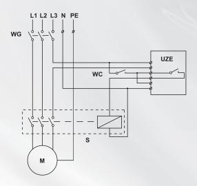
WG – main switch WC – pressure switch S – contactor M – motor
